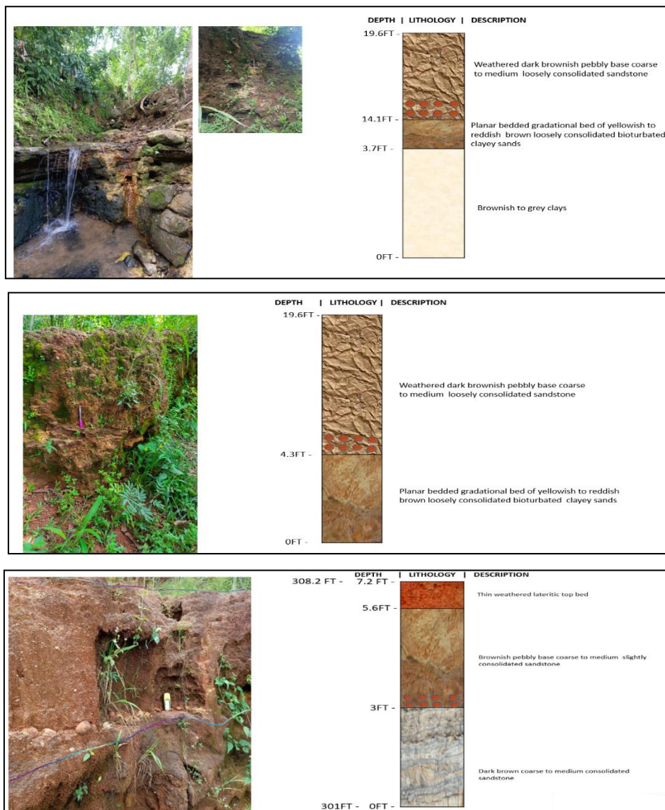
Figure 3a: (1) Field photograph and (2) stratigraphic log of Location 1a (Dennis Osadebay University Spring, Asaba) showing: (i) brownish to gray clays (0 – 3.7 ft), (ii) yellowish to reddish brown clayey sands (3.7– 14.1 ft) and (iii) weathered pebbly base loosely consolidated sandstones
