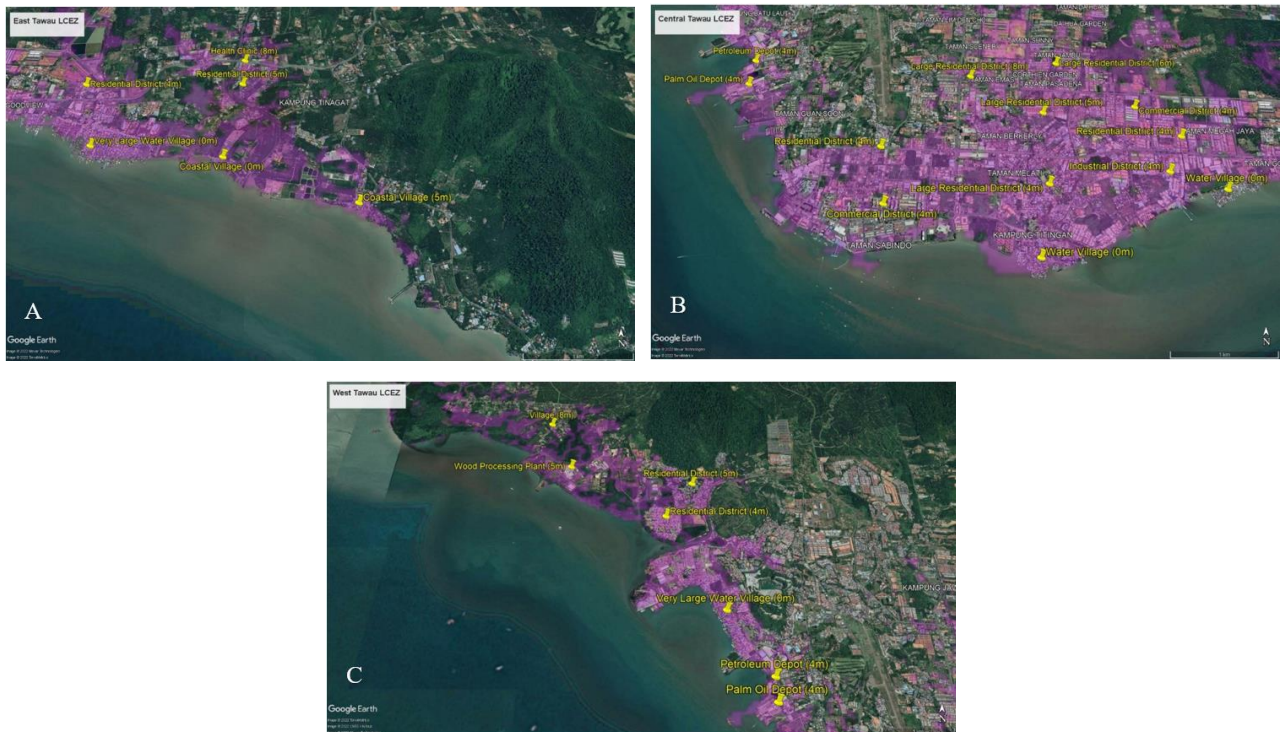
Figure 16: Tawau City LCEZ (magenta shading) derived from DEM data and depicted in GoogleEarth along with the identification of key vulnerable areas and constructions (yellow pins) to tsunami flooding. a) East Tawau City, b) Central Tawau City and, c) West Tawau City (Source: Author).
