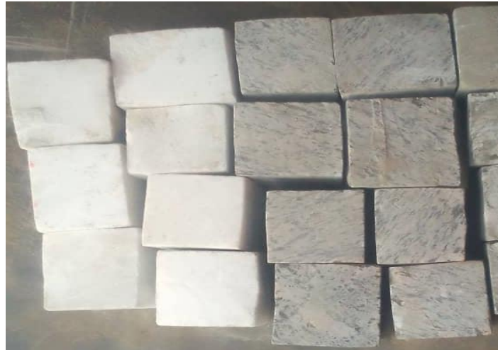
Figure 2: Rock samples used for unconfined compression test.
