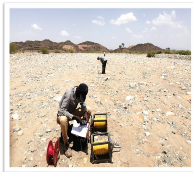
Plate 2: Schlumberger Array for VES measurement using SAS 1000, Red Sea State
