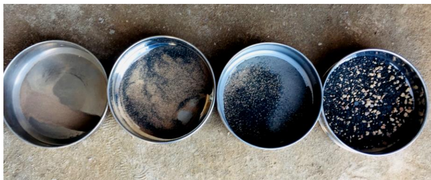
Figure 4: Sieve analysis test performed (Sieve no. 10, 40, and 200 were used).
