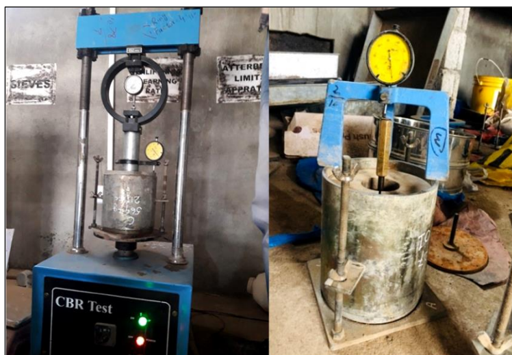
Figure 6: (a) Load vs penetration machine for CBR test (b) CBR mold with swell tripod.
