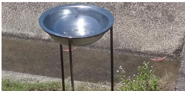
Figure 3: Rainwater collection stand
