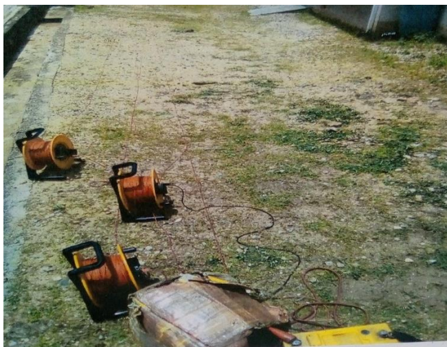
Plate 1: Material set up for the ERT survey.
