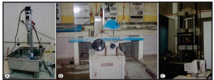
Figure 3: The coring machine, polishing and Hoek cell for triaxial test.
